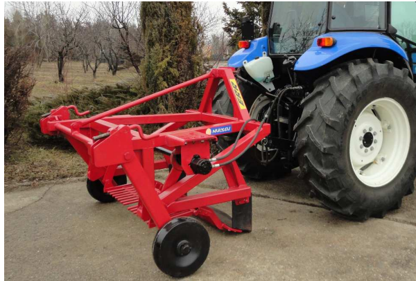
Fig. 3 - Technical equipment for harvesting the Miscanthus rhizomes ERR
